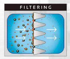
Wedge wire is a welded steel structure, mainly used for filtration, separation and retention media. It consists of surface profiles, usually V-shaped, that are resistance welded onto support profiles. The distance between the surface profiles is controlled very accurately, as it forms the slot through which the filtrate flows. In case of V-shapeed surface profiles conical slots are created (as shown on figure).
