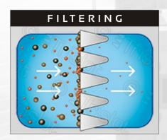
Wedge wire is a welded steel structure, mainly used for filtration, separation and retention media. It consists of surface profiles, usually V-shaped, that are resistance welded onto support profiles. The distance between the surface profiles is controlled very accurately, as it forms the slot through which the filtrate flows. In case of V-shapeed surface profiles conical slots are created (as shown on figure).
